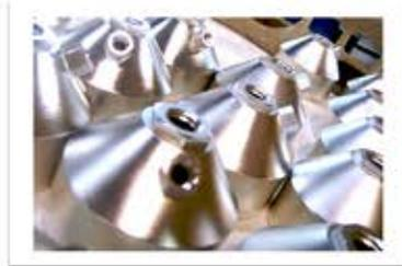
**RoHS Compliant** - AFT offers both traditional hexavalent Chemical Film and RoHS hex-free Chemical Film coatings. We have selected MacDermid Iridite NCP non-chrome Passivate, as this process has been developed in response to the ELV, RoHS and WEEE directives. Iridite NCP
